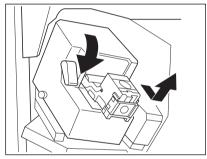
**3** Remove the empty staple case upward from the staple cartridge.
